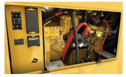
ENGINE. The TR6400 features a Cat C3.6L Tier 4F (Stage V), 99 hp (74.4 kW) engine. The engine is mounted on a pivoting frame that swings out 30 degrees for access to fuel filters and hydraulic reservoir for maintenance and service.
