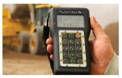
CONTROL SYSTEM. Operators can control the machine through either the Vermeer DP10 display mounted on the control panel, or through a handheld transceiver remote. From either control, the operator can choose from four programmable presets or adjust on the fly based on the incoming material.
