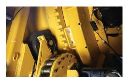
DRUM DRIVE. A hydraulic chain drive system allows the drum to lift off the cog for service. Bolt-on sprockets can be changed quickly and help minimize repair.
